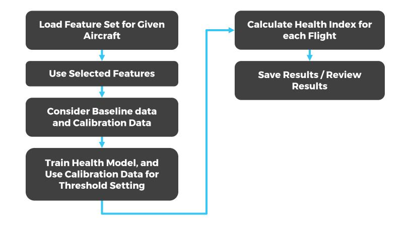
The idea behind this approach is to use these key features, and to build a multivariate health model that will provide an early indication of the emerging valve problem.
